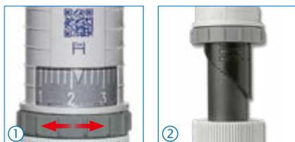
Large display is easy to read; the window adjusts to desired side of instrument body. Each step on the cylindrical cam is pre-calibrated and corresponds to one division on the volume adjustment scale.
